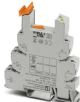
14 mm PLC basic terminal block for high continuous currents with screw connection, without relay or solid-state relay, for mounting on DIN rail NS 35/7,5, 1 changeover contact, input voltage 24 V AC/DC
