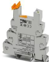
14 mm PLC basic terminal block for output functions with screw connection, without relay or solid-state relay, for mounting on DIN rail NS 35/7,5, with load return line connection (BB), 2 N/O contacts (1-1), input voltage 24 V DC
