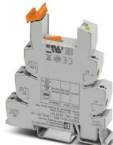
14 mm PLC basic terminal block with screw connection, without relay or solid-state relay, for mounting on DIN rail NS 35/7,5, 2 changeover contacts, input voltage 120 V AC/DC
