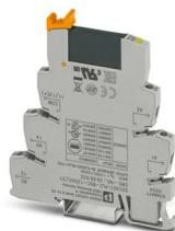
PLC-INTERFACE, consisting of PLC-BSC.../21 basic terminal block with screw connection and plug-in miniature solid-state relay, for mounting on DIN rail NS 35/7,5, 1 N/O contact, input: 120 V AC/110 V DC, output: 3 - 48 V DC/100 mA
