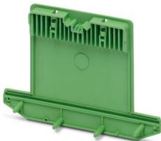
Side element, tall version, for closing both ends of the base element UM-BEFE, with guide grooves for vertically arranged printed circuit boards, for 73 mm wide U-shaped profile cover
