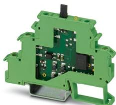
Input solid-state relay terminal block, input: 125 V DC, output: 3 - 48 V DC/100 mA, with isolating plug in output, terminal block width: 6.2 mm
