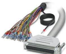
Assembled shielded round cable; connection 1: Single wires (37-position) (The wires are marked and fitted with ferrules. The braided shield is routed to a separate cable end.); connection 2: D-SUB socket strip (1x 37-position); cable length: 4 m
