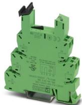
14 mm PLC basic terminal block for high continuous currents with spring-cage connection, without relay or solid-state relay, for mounting on DIN rail NS 35/7,5, 1 changeover contact, input voltage 230 V AC/DC
