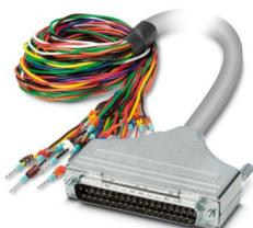
Assembled shielded round cable; connection 1: Twisted pair (37-position) (The wires are marked and fitted with ferrules); connection 2: D-SUB pin strip (1x 37-position); cable length: 30 m
