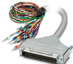
Assembled shielded round cable; connection 1: Single wires (37-position) (The wires are marked and fitted with ferrules); connection 2: D-SUB pin strip (1x 37-position); cable length: 30 m
