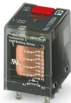
Plug-in industrial relay in basic design with power contacts, 4 changeover contacts, test button, status LED, mechanical switch position indicator, input voltage: 115 V AC
