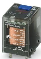
Plug-in industrial relay in basic design with power contacts, 4 changeover contacts, test button, status LED, mechanical switch position indicator, polarity A1+, A2-, input voltage: 125 V DC
