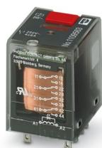
Plug-in industrial relay in basic design with power contacts, 4 changeover contacts, test button, status LED, mechanical switch position indicator, input voltage: 24 V AC
