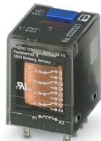
Plug-in industrial relay in basic design with power contacts, 4 changeover contacts, test key, mechanical switch position indicator, polarity A1+, A2-, input voltage: 24 V DC
