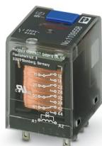
Plug-in industrial relay in basic design with power contacts, 4 changeover contacts, test button, status LED, mechanical switch position indicator, polarity A1+, A2-, input voltage: 48 V DC
