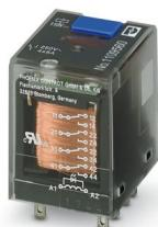
Plug-in industrial relay in basic design with power contacts, 4 changeover contacts, test button, status LED, mechanical switch position indicator, polarity A1+, A2-, input voltage: 110 V DC
