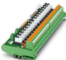
16-channel relay module for Honeywell C300 input modules. The module is controlled by the control system via 37-pos. D-SUB or 50-pos. FLK. A screw connection with knife disconnection is available in the field. Module width: 343 mm
