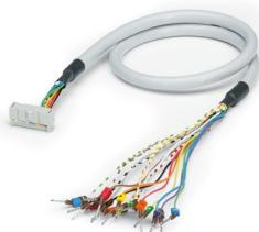
Assembled, shielded round cable with a 16-pos. socket strip and an open end. At the open end, the wires are labeled 1 to 16 and are fitted with ferrules, shield connection at open end, cable length: 27 m
