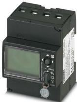
Three-phase energy meter for real power measurement in networks up to 460 V / 65 A, with 3 digital inputs and RS-485 interface, certified according to the MID directive
