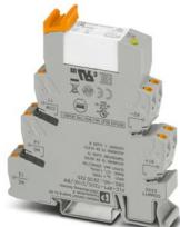
PLC-INTERFACE for railway applications and high continuous currents, consisting of basic terminal block with Push-in connection and plug-in miniature relay, range:  $0.7 \times U_N$  to  $1.25 \times U_N$ , temperature class TX:  $-40^\circ\text{C}$  to  $+70^\circ\text{C}$ , 1 changeover contact, input voltage 72 V DC
