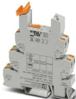
14 mm PLC basic terminal block with Push-in connection, without relay or solid-state relay, for mounting on DIN rail NS 35/7,5, 2 changeover contacts, input voltage 230 V AC/DC
