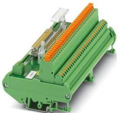
16-channel module with LED for Honeywell C300 modules. The module is controlled by the control system via 37-pos. D-SUB or 50-pos. FLK. A spring-cage connection (1+, 1-,...16+,16-) with knife disconnection is provided in the field. Module width: 170 mm
