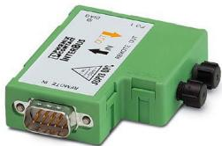
INTERBUS fiber optic adapter, for converting the remote IN interface to fiber optics, FO output left, correction of the optical transmission power
