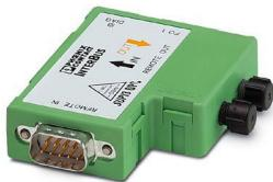
INTERBUS fiber optic adapter, for converting the remote IN interface to fiber optics, FO output right, correction of the optical transmission power
