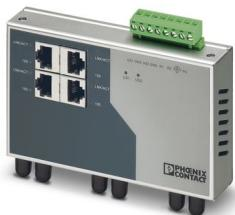
Ethernet switch, 4 TP RJ45 ports, 3 FO ports, 100 Mbps full duplex in ST-D format, automatic detection of data transmission speed of 10 or 100 Mbps (RJ45), auto crossing function
