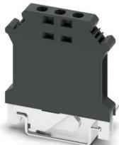
Reference potential terminal block, When aligning with a feed-through terminal block with the same shape, an end cover must be interposed with insulation voltages of > 690 V, number of connections: 2, number of positions: 1, connection method: Screw connection, Rated cross section: 4 mm<sup>2</sup>, cross section: 0.2 mm<sup>2</sup> - 4 mm<sup>2</sup>, mounting type: NS 35/7,5, NS 35/15, NS 32, color: black
