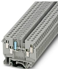
Component terminal block, nom. voltage: 630 V, nominal current: 32 A, number of connections: 4, connection method: Screw connection, Rated cross section: 4 mm<sup>2</sup>, 1 level, cross section: 0.2 mm<sup>2</sup> - 6 mm<sup>2</sup>, mounting type: NS 35/7,5, NS 35/15, NS 32, color: gray
