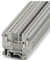
Component terminal block, for installing components that can be individually selected, nom. voltage: 630 V, nominal current: 32 A, number of connections: 4, connection method: Screw connection, Rated cross section: 4 mm<sup>2</sup>, 1 level, cross section: 0.2 mm<sup>2</sup> - 6 mm<sup>2</sup>, mounting type: NS 35/7,5, NS 35/15, NS 32, color: gray
