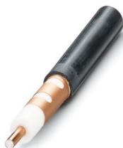
The 2.4 GHz leaky wave cable is a “wireless cable” that acts as an antenna and emits along its entire length. The range is limited. Track-guided systems, for example, can therefore be supplied as required, even under difficult conditions.
