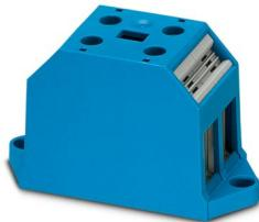
Device terminal block, nom. voltage: 630 V, nominal current: 150 A, number of connections: 4, connection method: Screw connection, Rated cross section: 35 mm<sup>2</sup>, cross section: 0.75 mm<sup>2</sup> - 50 mm<sup>2</sup>, mounting type: direct screw connection, color: blue
