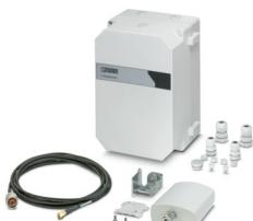
Control box set for constructing wireless systems for industrial applications, incl. panel antenna and 3 m antenna cable for 2.4/5 GHz, IP66, with DIN rail, plugs, and screw connections, with 100 V ... 240 V power supply unit, without devices
