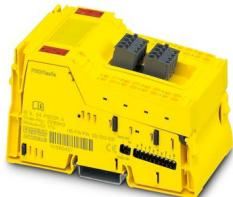
Safety-related distributed relay output module, IP20 protection, for the PROFIsafe system. The module has 4 safe relay outputs, each with two contacts. The output states are mirrored for diagnostic purposes.
