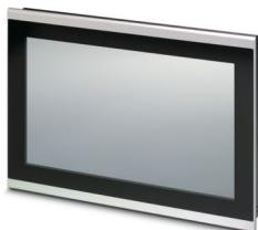
Touch panel, 30.7 cm / 12.1"-TFT display (projective-capacitive (PCAP)), 1280 x 800 pixel(s) (WXGA), 65536 colors, Arm® Cortex®-A8, 1000 MHz, 2x USB Host 2.0, 1 x Ethernet (10/100 Mbps), RJ45, Windows® Embedded Compact 7, Movicon™, without bus system.
