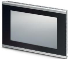
Touch panel, 17.8 cm / 7"-TFT display (projective-capacitive (PCAP)), 800 x 480 pixel(s) (WVGA), 16.7 million colors, Arm® Cortex®-A8, 1000 MHz, 2x USB Host 2.0, 1 x Ethernet (10/100 Mbps), RJ45, Windows® Embedded Compact 7, IniNet Browser, without bus system.
