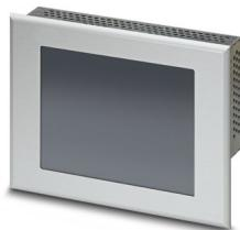
Touch panel, 14.5 cm / 5.7"-TFT display (analog resistive (polyester)), 320 x 240 pixel(s) (QVGA), 65536 colors, Arm9™, 200 MHz, 1x COM (RS-232/485), 1 x Ethernet (10/100 Mbps), RJ45, Windows® CE 5.0 Professional, TSvisRT, without bus system.
