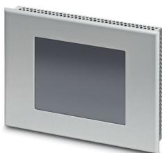
Touch panel, 14.5 cm / 5.7"-FSTN display (analog resistive (polyester)), 320 x 240 pixel(s) (QVGA), 5 grayscales, Arm9™, 200 MHz, 2x USB Host 2.0, 1 x Ethernet (10/100 Mbps), RJ45, Windows® CE 5.0, TSvisRT, CAN.
