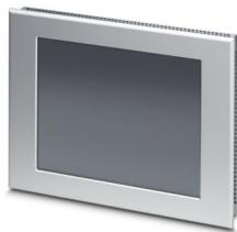
Touch panel, 26.4 cm / 10.4"-TFT display (analog resistive (polyester)), 800 x 600 pixel(s) (SVGA), 262144 colors, Arm® Cortex®-A8, 800 MHz, 2x USB Host 2.0, 1 x Ethernet (10/100 Mbps), RJ45, Windows® Embedded Compact 7, Open platform, without bus system.
