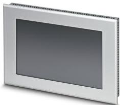
Touch panel, 22.9 cm / 9"-TFT display (analog resistive (polyester)), 800 x 480 pixel(s) (WVGA), 16.7 million colors, Arm® Cortex®-A8, 800 MHz, 2x USB Host 2.0, 1 x Ethernet (10/100 Mbps), RJ45, Windows® Embedded Compact 7, Open platform, without bus system.
