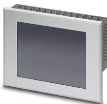
Touch panel, 14.5 cm / 5.7"-TFT display (analog resistive (polyester)), 640 x 480 pixel(s) (VGA), 262144 colors, Arm® Cortex®-A8, 800 MHz, 2x USB Host 2.0, 1x COM (RS-232), 1x COM (RS-422/485), 1 x Ethernet (10/100 Mbps), RJ45, Windows® Embedded Compact 7, Open platform, DualCAN.
