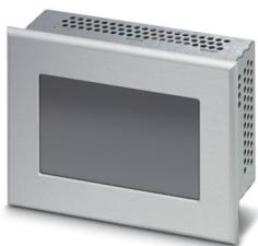
Touch panel, 10.92 cm / 4.3"-TFT display (analog resistive (polyester)), 480 x 272 pixel(s) (WQVGA), 262144 colors, Arm® Cortex®-A8, 800 MHz, 2x USB Host 2.0, 1 x Ethernet (10/100 Mbps), RJ45, Windows® Embedded Compact 7, Movicon™, without bus system.
