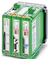
PROFIBUS DP to PROFIBUS PA coupler system for integration and diagnostics of PROFIBUS PA in PROFIBUS DP. Includes the one-network head station unit (FB-HSB), PROFIBUS DP repeater with oscilloscope (FB-DP-RPTR/SC), and PROFIBUS PA interface module with oscilloscope.
