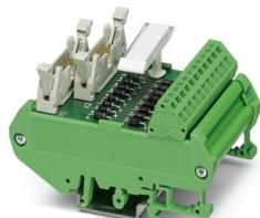
VARIOFACE interface module for redundant connection of 2x8 output channels (SIMATIC® S7 / S5) via 2xFLK14 on spring-cage terminal blocks, signals are decoupled by diodes
