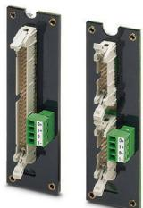
VARIOFACE front adapters, for ControlLogix, max. 1 x 32 channels can be connected, number of positions 50.
