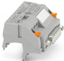
V8 adapter for 8 x PLC-INTERFACE (6.2 mm), controller: PLC system cabling of output cards, connection 1: D-SUB socket strip 1x 15-position, connection 2: Plug-in connection (Can be snapped onto 8x PLC-INTERFACE terminals), connection 3: Screw connection 1x 2-position, number of channels: 8, control logic: positive switching
