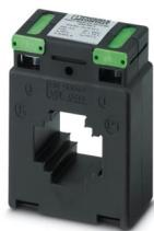
Window-type current transformer, 250 A AC primary current; 5 A AC secondary current; accuracy class 1; 5 VA rated power
