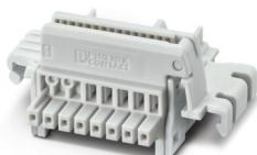
DIN rail bus connector, color: light gray, nominal current: 6 A, 4 A (parallel contacts) (Serial contacts), rated voltage (III/2): 32 V, number of positions: 8, product range: TBUS8-20.., pitch: 2.54 mm, mounting: DIN rail mounting, locking: without, mounting method: without, type of packaging: packed in cardboard, Item with gold-plated contacts, bus connectors for connecting with electronics housings, 6 parallel contacts/2 serial contacts
