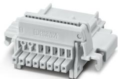
DIN rail bus connector, color: light gray, nominal current: 6 A (parallel contacts), rated voltage (III/2): 32 V, number of positions: 8, product range: TBUS8-25.., pitch: 2.54 mm, mounting: DIN rail mounting, locking: without, mounting method: without, type of packaging: packed in cardboard, Item with gold-plated contacts, bus connectors for connecting with electronics housings, 8 parallel contacts
