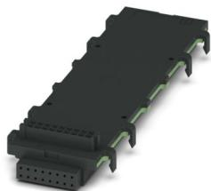
DIN rail bus connector, color: black, nominal current: 3 A (Total current of 25 A max.), rated voltage (III/2): 30 V, number of positions: 16, product range: BC 107,6.., pitch: 2.54 mm, mounting: DIN rail mounting, locking: without
