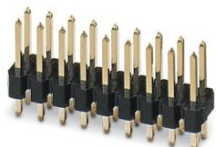
Pin strip, color: black, contact connection type: Pin, number of potentials: 18, number of rows: 2, number of positions: 18, number of connections: 18, product range: PSTD 0,65X0,65/..-V, pitch: 2.54 mm, mounting: THR soldering, pin layout: Linear pinning, solder pin [P]: 2.5 mm, locking: without, type of packaging: packed in cardboard
