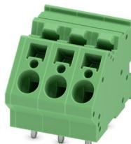
Printed circuit board terminal, nominal current: 32 A, rated voltage (III/2): 630 V, nominal cross section: 4 mm<sup>2</sup>, number of potentials: 3, number of rows: 1, number of positions per row: 3, product range: ZFKDS(A) 4, pitch: 7.5 mm, connection method: Spring-cage connection, mounting: Wave soldering, conductor/PCB connection direction: 45 °, color: green, Pin layout: Linear pinning, Solder pin [P]: 4.6 mm, number of solder pins per potential: 2, type of packaging: packed in cardboard
