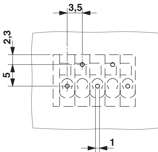
The figure shows the drilling plan of the 5-pos. version of the article – Zig-zag pinning starts at the right-hand position. Other pinning available on request.
