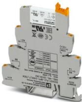
PLC-INTERFACE for input functions, consisting of PLC-BPT.../SEN basic terminal block with push-in connection and plug-in miniature relay with multi-layer gold contact, for mounting on DIN rail NS 35/7,5, 1 N/O contact, input voltage 24 V DC
