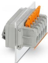
Panel feed-through terminal block, connection method: Push-lock connection, Push-in spring connection, number of positions: 4, load current: 41 A, cross section: 2.5 mm<sup>2</sup> - 16 mm<sup>2</sup>, connection direction of the conductor to plug-in direction: 0 °, width: 64.4 mm, color: gray
