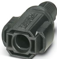
Photovoltaic connector, Range of articles: SUNCLIX, color: black, number of positions: 1, rated voltage: 1000 V DC, rated current: 40 A, Connection method: Crimp
