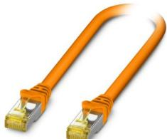
Patch cable, RJ45/IP20 straight on RJ45/IP20 straight, cable length: 20 m, number of positions: 8, 10 Gbps, CAT6<sub>A</sub>, connection cross section: AWG 26- 26, Ethernet, 4x2xAWG26/7; S/FTP, orange
