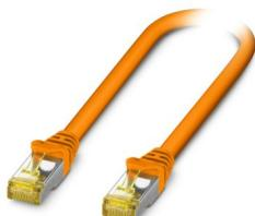
Patch cable, RJ45/IP20 straight on RJ45/IP20 straight, cable length: 5 m, number of positions: 8, 10 Gbps, CAT6<sub>A</sub>, connection cross section: AWG 26- 26, Ethernet, 4x2xAWG26/7; S/FTP, orange
